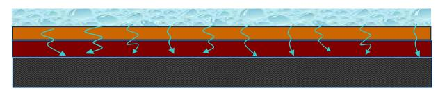
**3** CRC active components then induce "stress" on the chemical bonds of the coating, and reaction separates coating from substrate
